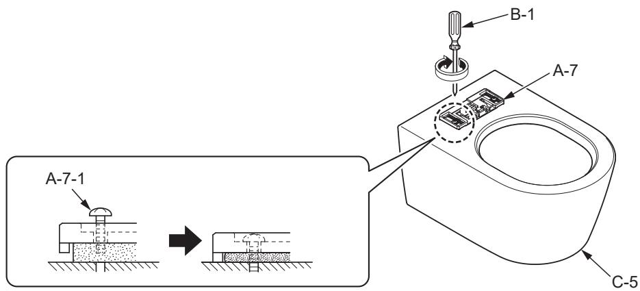
Failure to tighten screw A-7-1 completely will cause moving sideways of C-1.
